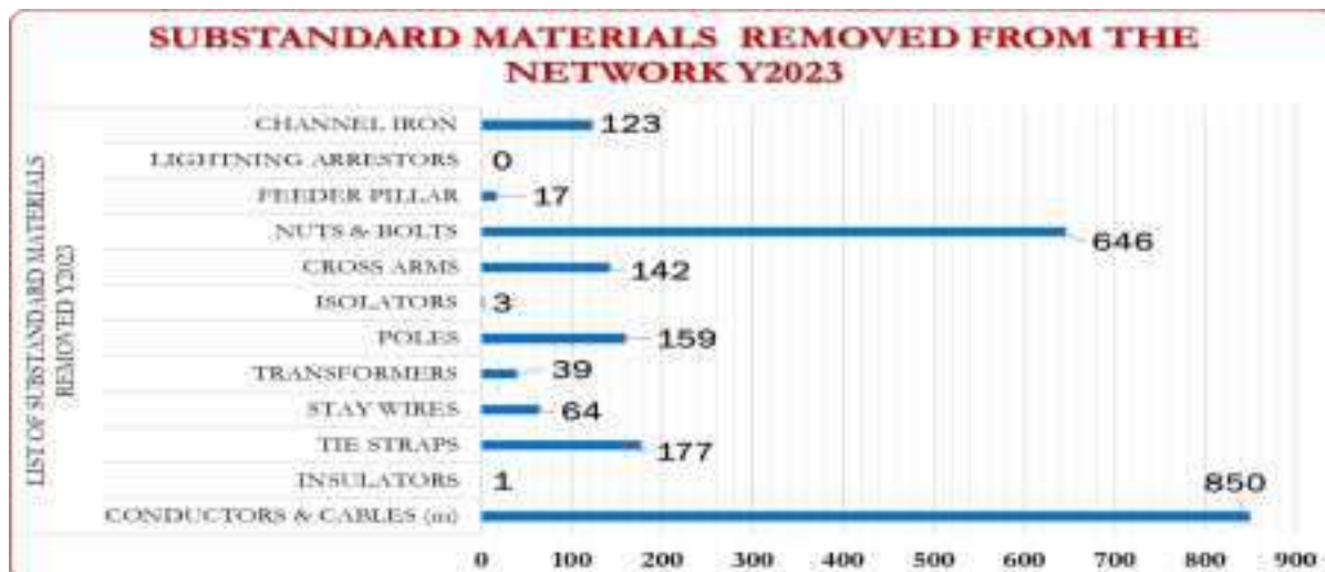
Figure 3: Substandard electrical materials/ equipment removed from system in year 2023
