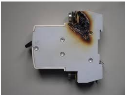
Figure 4: Broken Circuit Breaker
